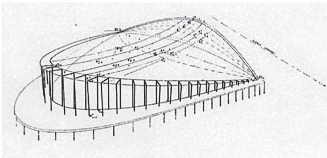
Fig. 2: Unrealised project (1951) by Laffaille for roofing the CIM (Centre of the Mechanical Industries) with a steel membrane or steel cables (Nogue, 2004, 195).
