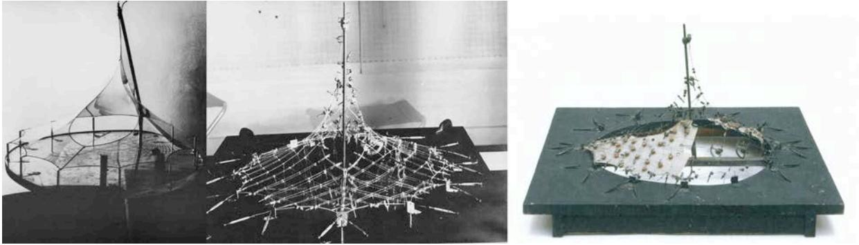
Figure 4-6: *Institut für Leichte Flächentragwerke* Stuttgart, IL-Pavillon 1966-1967, form-finding soap-film model, physical model 1965 double-exposure shot, the preserved model 2012 (IL 18, p. 477/saai Karlsruhe/DAM Frankfurt)
