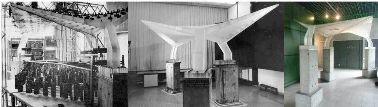
Figure 1-3: *Institut für Modellstatik* Stuttgart, “Alster-Schwimmhalle” swimming baths Hamburg 1956-1972, physical model, under load, the preserved model 2014 (saai Karlsruhe/photo Johanna Moosmann 2014)
