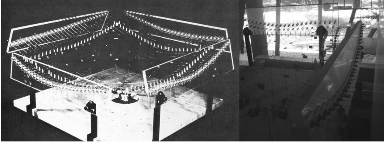
Figure 7-8: *Institut für Leichte Flächentragwerke* Stuttgart, detail physical model of the low-point of the swimming arena for the Olympic Games 1972 Munich, the published model and the preserved model 2014 (IL 8, p. 297/photo Daniel Klausner 2014)
