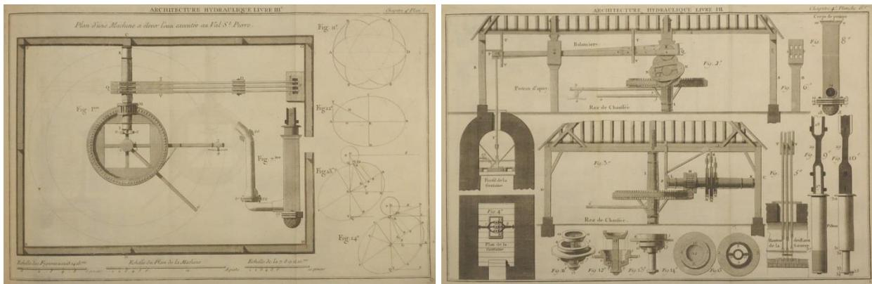
Figures 6 and 7: Water lifting machine as built in the Chartreuse en Tiérache, val Saint-Pierre, near Vervins, France, plan, sections and details; from: Bélidor 1739, 3<sup>rd</sup> book, 4<sup>th</sup> chapter, plans 5 and 6 (Bibliotheca Hertziana)
