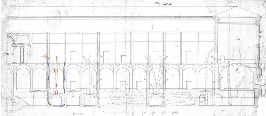
Figure 3: Alte Pinakothek Munich, Section drawing illustrating the warm air ducts (red arrows) and exhaust air ducts (blue arrows) of the air heating system, 1825 (Architekturmuseum der TU München)
