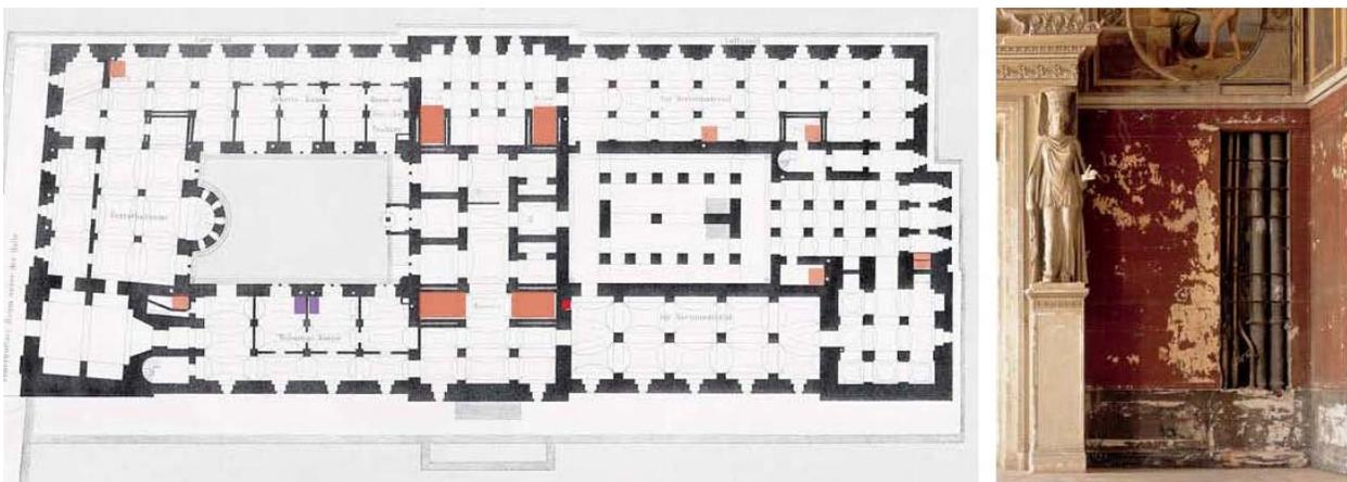
Figure 4: Neues Museum, left – basement floor plan indicating the location of the boilers for the hot water heating (red), the air heating ovens (light red) and the local ovens (violet), 1853 (Architekturmuseum TU Berlin); right – oval smoke flues for the hot water heating in the north wall of Niobid Room, 2003 (J.v. Bruchhausen, Berlin)
